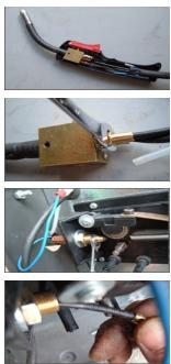
The torch comes apart with 4 screws. Inside this one there is a brass block that switches the flow of shielding gas (many other welders have an electrical solenoid inside the machine to switch the gas).
