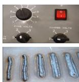
It's worth knowing that the wire speed also controls the amps.
