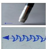
The contact tip should be about 6mm to 10mm from the metal to be welded, so cutting the wire about 10mm long and holding the torch so the wire touches the sheet is a good way to position a MIG welder.
