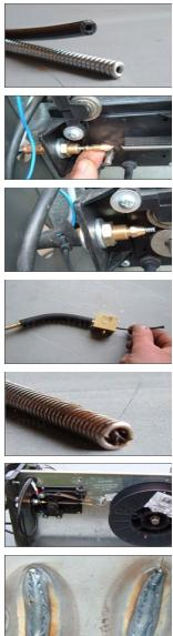
The swan neck won't normally need to be replaced unless the screw thread for the tip is damaged, but it's a quick and easy job. The neck is clamped into the brass block with a grub screw.
